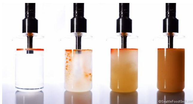
Figure 1-3 Effect of Ultrasonic in Homogenization
