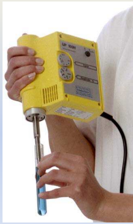
UP100H - compact light-weight ultrasonic device
