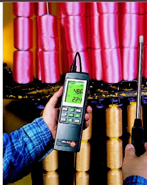
Humidity measurement up to +180^\circ\text{C} in drying systems
