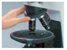
lengths and longer working distances provide more working space around the nosepiece.
