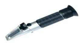
The MT-200 is designed to measure the protein levels in blood serum. It works great for checking the protein levels in lobster blood to assure the quality is good.
