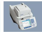
2003 Mastercycler ep: Fast heating/cooling rates and ultra quiet operationin a compact design.
