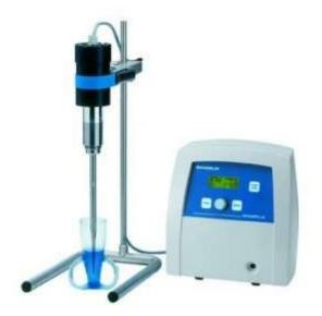
SONOPULS homogenisers with integrated amplitude control 10-100 % and actual value display, pulsation, AMPLICHRON®-System, built-in timer, remote controlled. CE-marked, also as medical device compliant to the directive for in-vitro diagnostics 98/79/EG. HD 3100, HD 3200 und HD 3400 with power control, temperatur and energy monitoring, 9 user programs and PC control.
